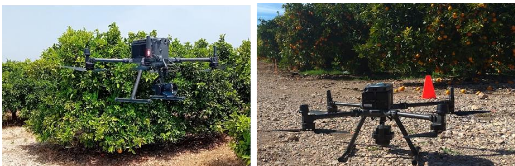
Figure 2.2 M350 RTK drone in orange orchards: Sony RGB camera (Left) and LiDAR sensor (Right).
