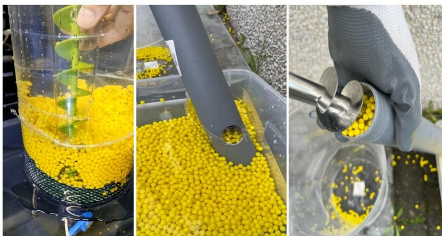
Figure 4.3. First test of the cochlea using plastic beads.
