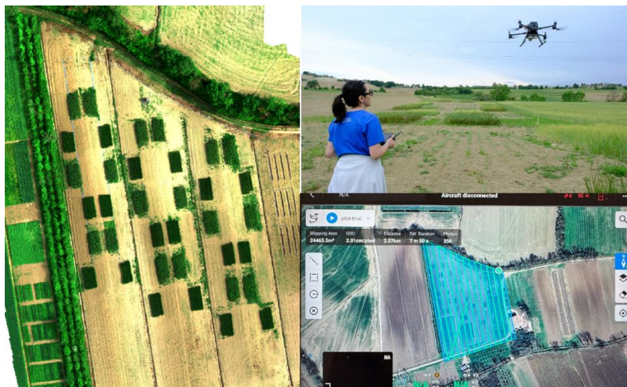
Figure 3.2 Orthomosaic of the trial plots, details of the flight using the DJI Matrice 350 RTK drone, and the flight plan over the plots trial.
